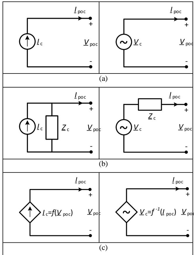
Figure 7 Different model structures of PGUs: (a) Independent current and voltage sources, (b) Norton and Thévenin equivalent circuit, (c) Dependent current and voltage sources
