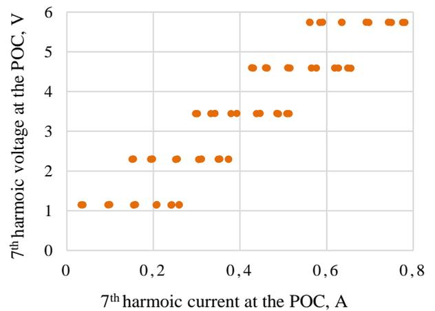
Figure 8 Test-bench measurement results (harmonic voltage-current pairs at the POC) on a small photovoltaic power generation unit
