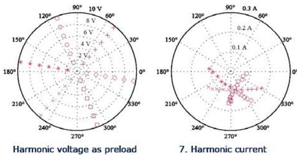
Figure 4 Fingerprint method, where harmonic voltages, varying in amplitude and phase are given as a preload to the inverter, which then reacts with a harmonic current. This example shows the current for the 7th harmonic.
