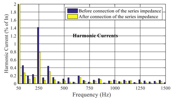
Figure 6 Influence of the grid impedance on the harmonic emission of a PGU (blue: low grid impedance, yellow: high grid impedance).
