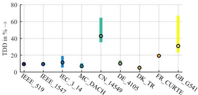
Figure 12 Total demand distortion (TDD) of methods for generating installations in low voltage LV levels (5th to 95th percentile and median (black dot) for 100.000 sample installations)
