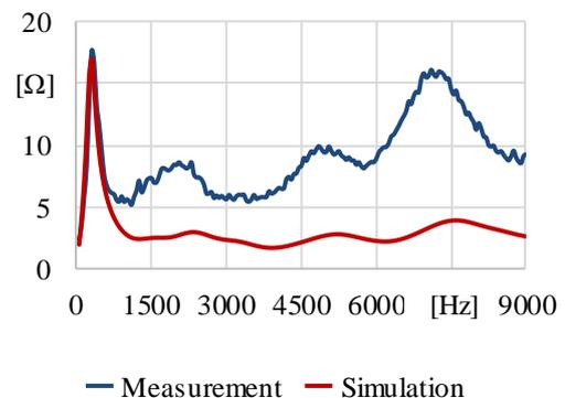
Figure 10 Frequency scan of measured and simulated harmonic impedance
